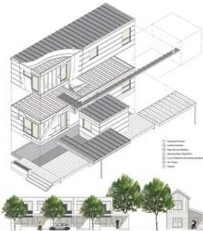
The Ability House concept centers on flexibility. The base module is a one-story, one-bedroom residence. With the addition of other modules, a family could construct a two- to four-bedroom, two-story house in two stylistic variations.
